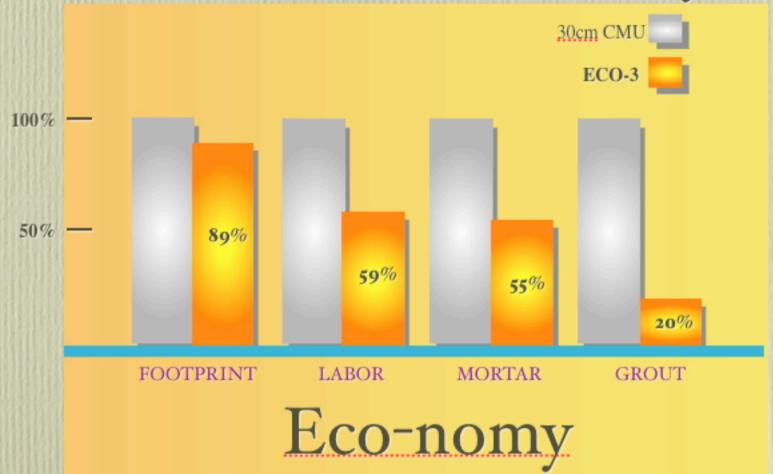
Footprint reduction due to increased wall slenderness. Labor reductions of 25 to 40% (depending on wall thickness) resulting from higher installation productivity. Mortar volume decrease from shorter jointing allowed by hybrid interlock. Grout volume substantially reduced by fractional area of dedicated cavity in EcoBloQ<sup>TM</sup>.
